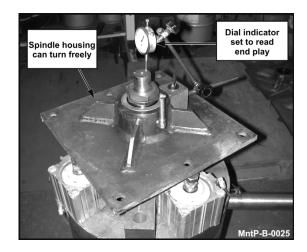
5. After the lock nut is tightened, there must be .001 inch to .003 inch of free play when lightly prying up on the spindle housing.
