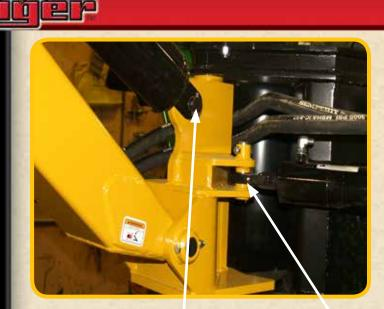
Connect boom arm cylinder to top tab on swivel. Connect swing cylinder with vertical pin located on right side of swivel.
