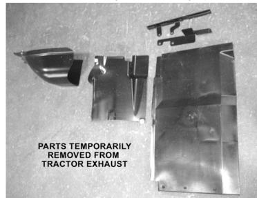
When removing heat shield parts from the tractor exhaust, save all hardware to re-install the heat shield after the John Deere tube bracket has been replaced
