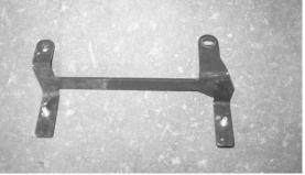
John Deere bracket to be replaced
