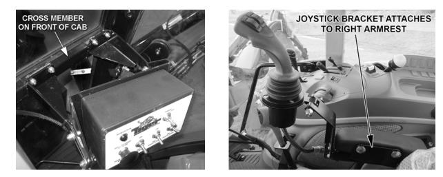
After installation of switchbox brackets 06411086, apply clear RTV (silicon) seal all around the outside of the bracket to prevent leaks.
