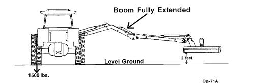
If the unit is operated on slopes greater than 5°, additional counterweight will be required. Operation of the unit on slopes greater than 11 percent (6.4 degrees) is not recommended under any circumstances. On a tractor with a 96" outside to outside tire spread, an 11 percent (6.4 degrees) slope occurs when one rear tractor tire is about 8" lower than the other rear tire. *OPS-B- 0018*
