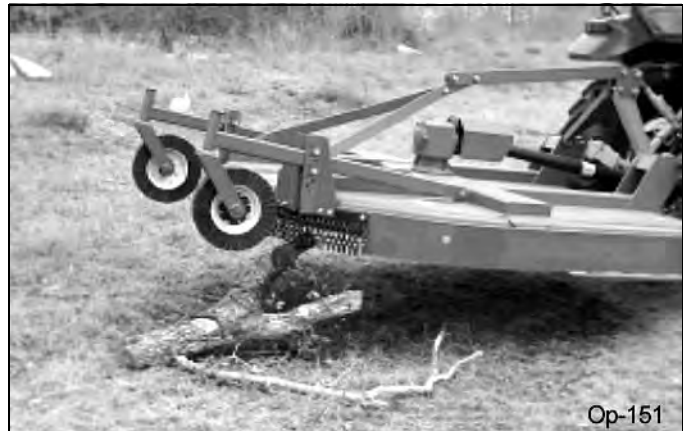
Raise Mower over solid objects
