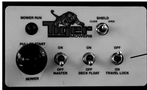
ELECTRONIC LIFT VALVE SWITCH BOX
