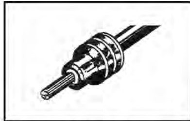
2. Align seal with cable insulation.
