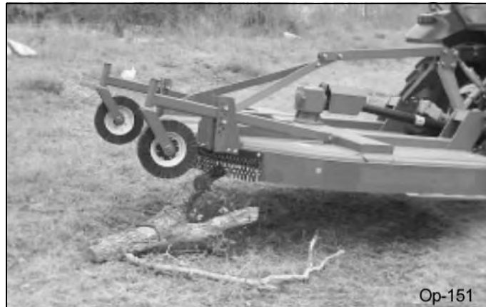
Raise Mower over solid objects
