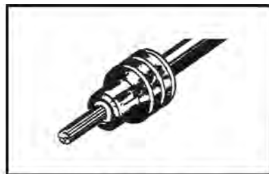
2. Align seal with cable insulation.
