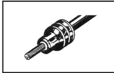
2. Align seal with cable insulation.
