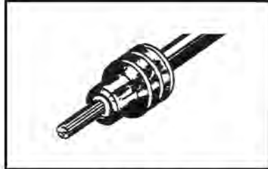
2. Align seal with cable insulation.
