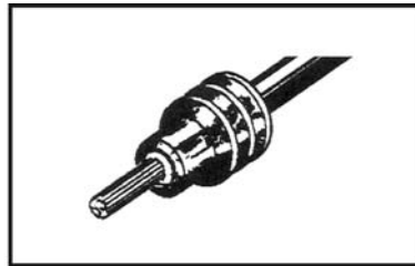
2. Align seal with cable insulation.
