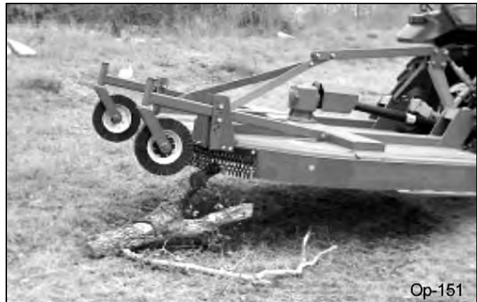
Raise Mower over solid objects
