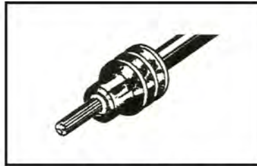
2. Align seal with cable insulation.
