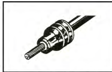
2. Align seal with cable insulation.
