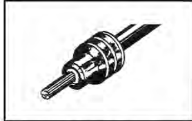
2. Align seal with cable insulation.
