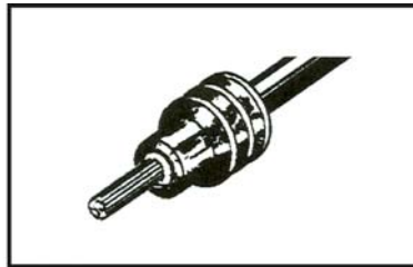
2. Align seal with cable insulation.
