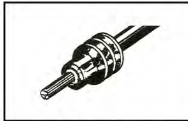
2. Align seal with cable insulation.
