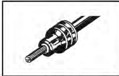
2. Align seal with cable insulation.
