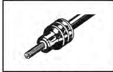
2. Align seal with cable insulation.
