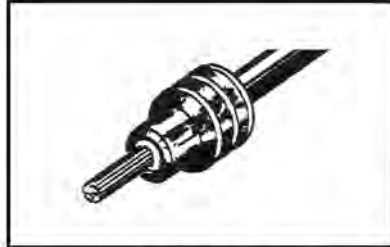
2. Align seal with cable insulation.
