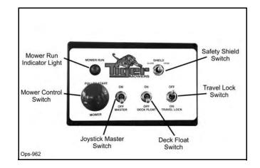
The Safety Shield switch opens and closes the shield located on the front of the cutter head. When moving at or near the ground, always have the shield in the closed position. When moving in brush or in trees above ground level the shield may be opened for easier cutting. Read and follow the warnings on the decal shown below. **Do not run the cutter into material larger than 6**" diameter.
