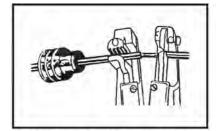
1. Apply seal to cable, before stripping insulation.
