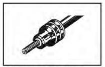
2. Align seal with cable insulation.
