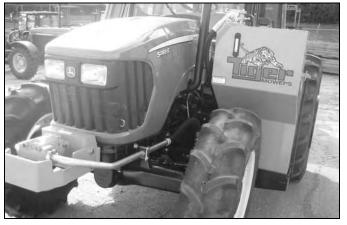
Check the fluid level in the Hydraulic Tank on the
