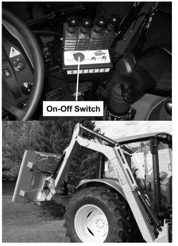
secondary boom contracts the side of the boomrest saddle. Next, slowly extend the knuckle cylinder until the secondary sets on the bottom part of the boomrest saddle.
