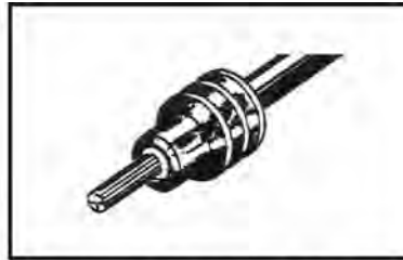
2. Align seal with cable insulation.
