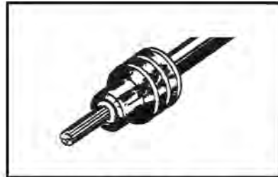
2. Align seal with cable insulation.
