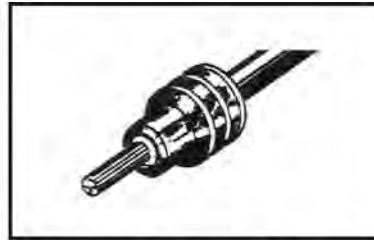
2. Align seal with cable insulation.
