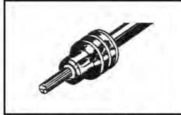
2. Align seal with cable insulation.
