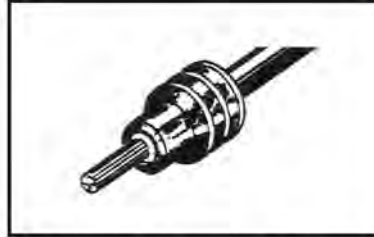
2. Align seal with cable insulation.
