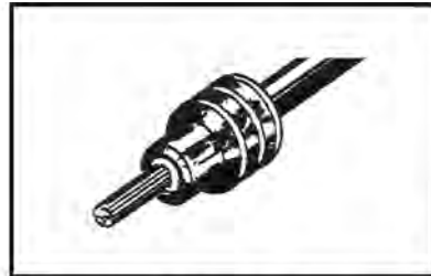
2. Align seal with cable insulation.
