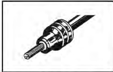
2. Align seal with cable insulation.
