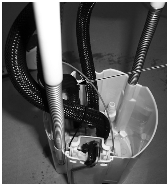
SENDING UNIT AFTER MODIFICATION
