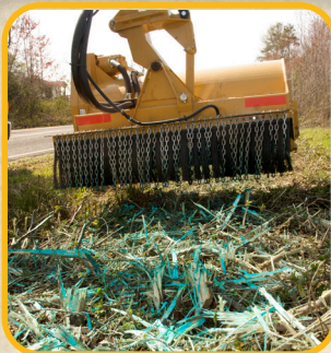
Spray Chamber attaches to Boom Flail Cutter Head.
