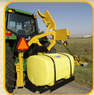
50, 100 & 150 gallon Tank mix systems are available for the tractor 3 PT hitch.
