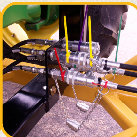
Plug & Play Bulkhead for quick disconnect
