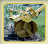
**DITCHER**22" diameter cutting width
