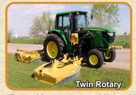
Twin Rotary Mowers come in 60" and 72" sizes for side and 60" rear.
