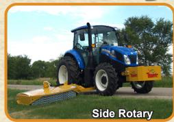
TSR Series domed top rotary cutters help to shed debris while cutting vegetation.
