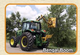
Bengal Booms - Rotary or Flail head in several sizes and Boom lengths of 18' to 24'.
