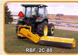
RBF 2C Series - designed with a 90° transport position and 50° degree below horizontal working position for steep slopes.
