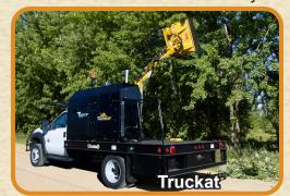
Truckat is a Boom Mower mounted to a HD truck bed. Cuts brush and grass, then drive quickly to your next job site.
