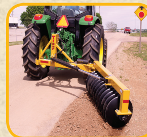
Patented angle design effectively moves and mulches 37" of material.
