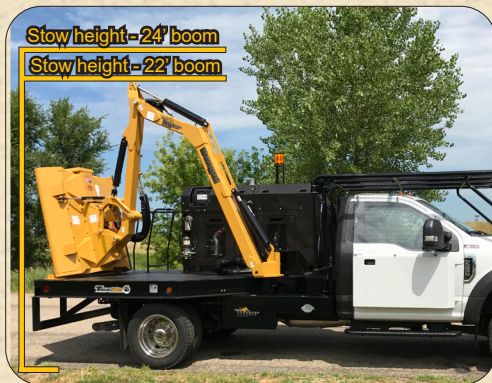
Stow Height - 13' 5" for 24' Boom Stow Height - 11' 8" for 22' Boom
