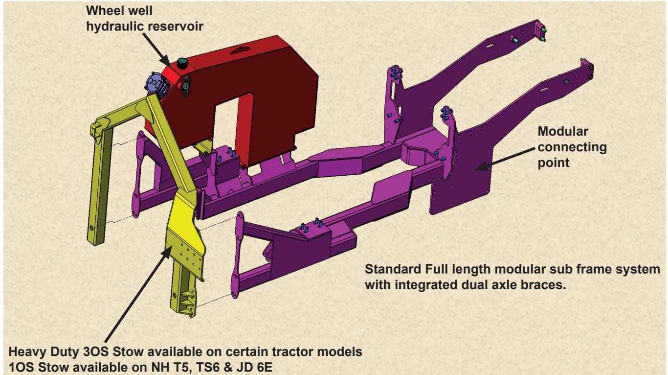
To enhance the adaptability of our products, Tiger offers a modular mounting frame to ease mower change for your vegetation needs. This unique design offers interchangeability from the Wildkat to any Tiger side mower system. (tractor remotes would be used for side mower)
